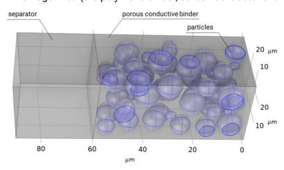
same domain) porous binder conductive and electrolyte phase. The anode is not explicitly included in the model but only implicitly through a boundary condition on the left side of the separator. The boundary condition on the right side of the cathode represents the current collector where inward electrode current is applied.
